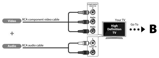
Supplied cables used in this connection are as follows: • RCA audio cable (L/R) x 1
